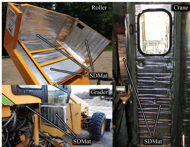
Fig. 3: Cabin and engine compartments with sound dampening mats installed
