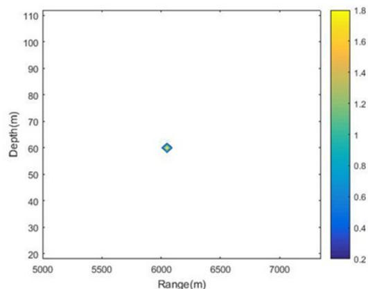
Fig. 8: Riemannian ambiguity surface for 20 modeled field replicas and 10 data replicas,  $SNR=-3dB$ , No of snapshot > 20 sample in 2 dimensions.
