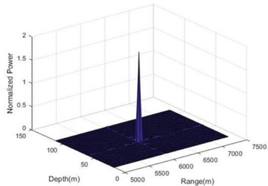
Fig. 7: Riemannian ambiguity surface for 20 modeled field replicas and 10 data replicas,  $SNR=-3dB$ , No of snapshot > 20 sample in 3 dimensions
