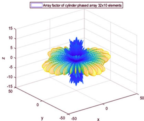
Fig. 5. The array factor of cylindrical hydrophone array of 32x10 elements. The result is reproduced from [10]
