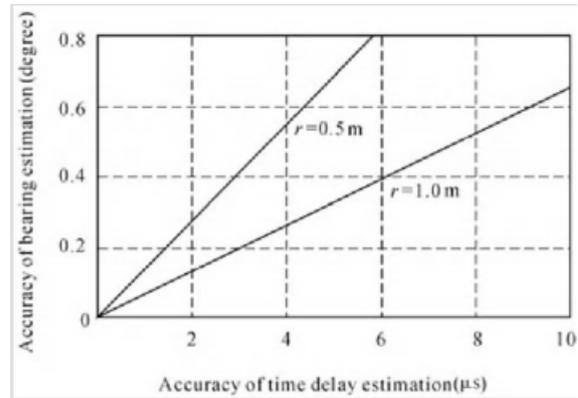
Fig. 6 Bearing accuracy of circle array ( $N=64$  elements). The result is reproduced from [11].
