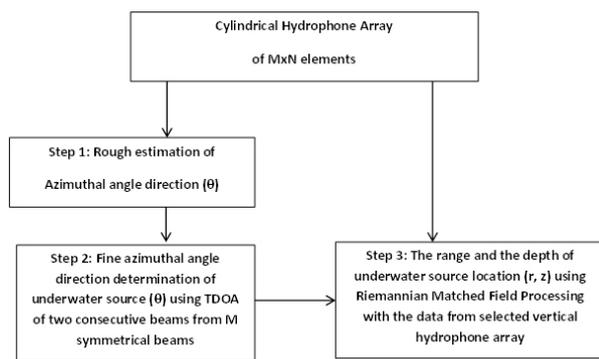
Fig. 2: The procedure of finding the azimuthal angle direction, the range and the depth of underwater source  $(\theta, r, z)$
