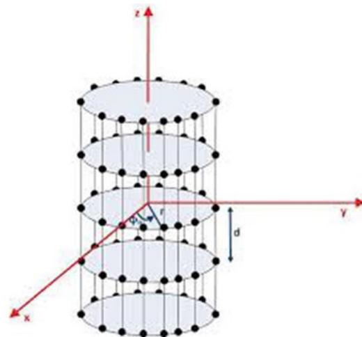
Fig. 1: The geometry of cylindrical hydrophone array of MxN elements (each ring has M elements)
