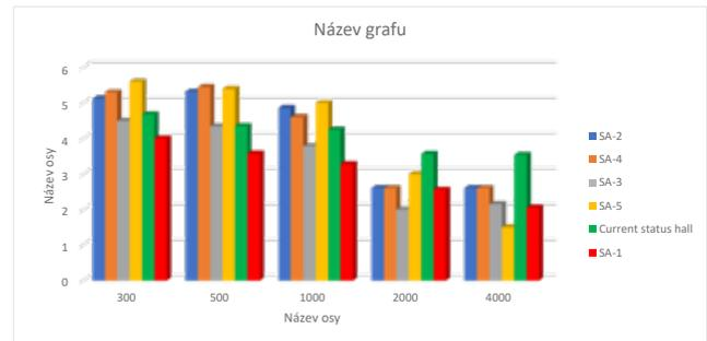
Fig. 3: Comparing the RT for different Model panels (SA1 to SA5) as simulated for the Airport Hall. The green data shows the current status of RT in the Airport Hall at frequencies 300-4000 Hz
