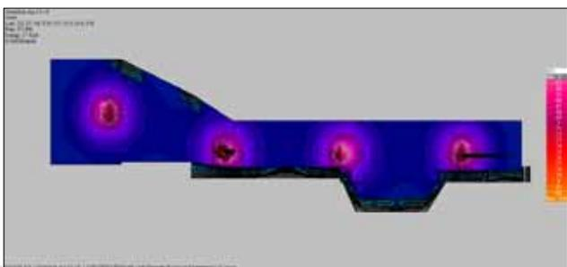
Fig. 7: Illustrating the simulation of STI the after installation of panels Model SA-1. The graphical contours represent sound from public hypothetical talkers
