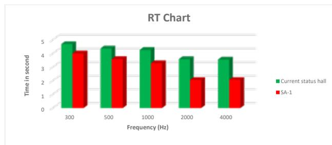
Fig. 4: Comparing the RT of current status Hall of Ahvaz Airport (Green color) to the virtual design square panels Model SA-1 (red color) in Frequencies from 300 Hz to 4000 Hz
