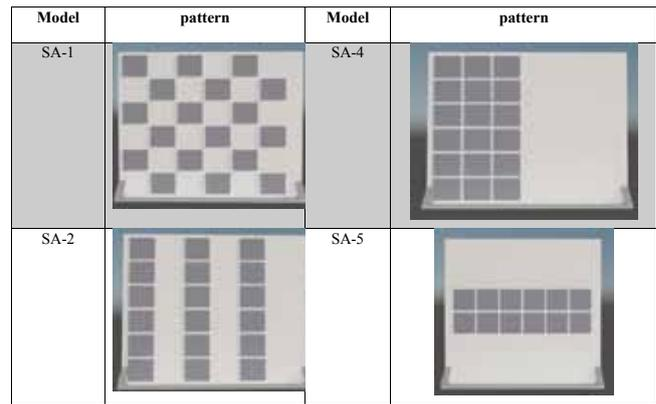
Fig. 1: Introducing the models (SA-1 to SA-5), each with a different pattern. The area of a single square panel is 0.115 by 0.115 meters.
