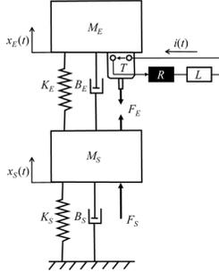
Fig. 1: Vibrating structure with semi-active vibration absorber
