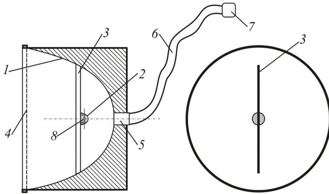
Fig. 1: General arrangement of the sonic flow densifier for auscultation purposes. 1 – parabolic reflector; 2 – reduced parabolic reflector; 3 – support; 4 – protective shield; 5 – center hole; 6 – sound duct; 7 – earpiece; 8 – parabolic reflector focus point
