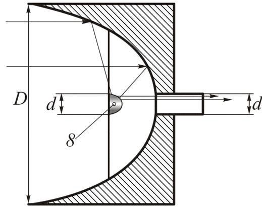
Fig. 2: Arrangement of the sonic flow densifier.  $D$  – entry sonic flow diameter;  $d$  – exit sonic flow diameter and reduced parabolic reflector diameter; 8 – parabolic reflector focus point
