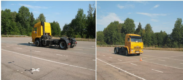
Fig. 8: Testing the muffler at a FSUE “NAMI” testing ground
