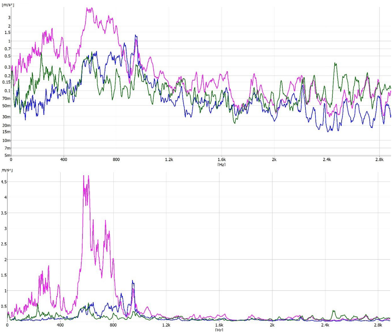
Fig. 3: Frequency spectrum in logarithmic and linear scales at the input of the primary suspension (6) and the outputs of the bogie pivot (10) and side bearer (9) into the tank shell at a speed of 120 km/h.
