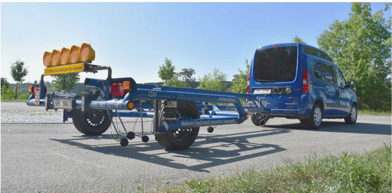
Fig. 1: Specialised CDV trailer for CPX measurements (source: CDV).
