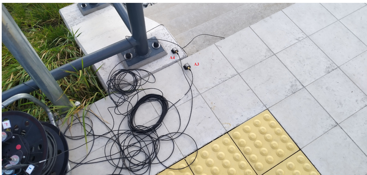
Fig. 4 The placement of vibration acceleration sensors on the platform
