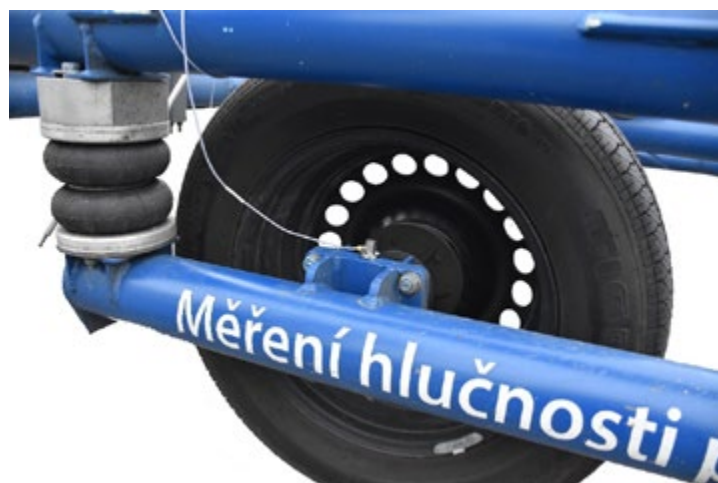
Fig. 3: Accelerometer location on the CPX measuring trailer.
