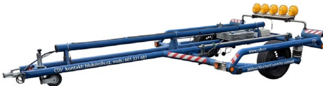
Fig. 1: Measuring trailer for CPX measurement.
