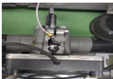
Fig. 3: Different measurement locations of the accelerometers of the analyzed bearing using a grub screw resting directly on the outer ring of the headstock bearing (left), on the frame using a grub screw (center), fixing with a magnet on the support frame of the drive unit under the analyzed bearing (right)
