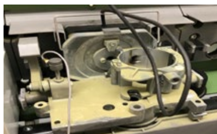
Fig. 3: Different measurement locations of the accelerometers of the analyzed bearing using a grub screw resting directly on the outer ring of the headstock bearing (left), on the frame using a grub screw (center), fixing with a magnet on the support frame of the drive unit under the analyzed bearing (right)
