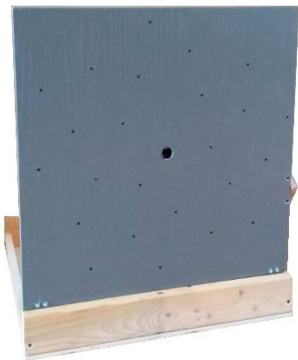
Fig. 5. Baseline logarithmic spiral array with a diameter of 0.59m
