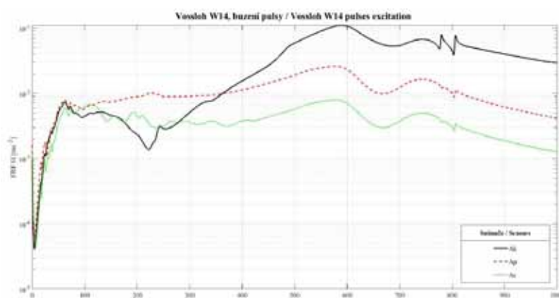
Fig. 6: Frequency transfer functions, excitation of the sample with a series of pulses
